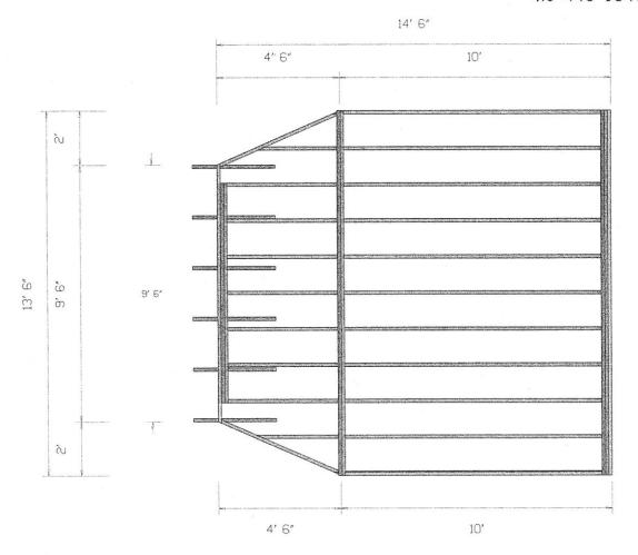
SITE DESCRITPION: The decking is 8.75" above ground level, and has no supporting posts. The ground is assumed to be level. Your deck will support a 105 PSF live load. Joists are to be placed on top of beams. 16" center to center.
