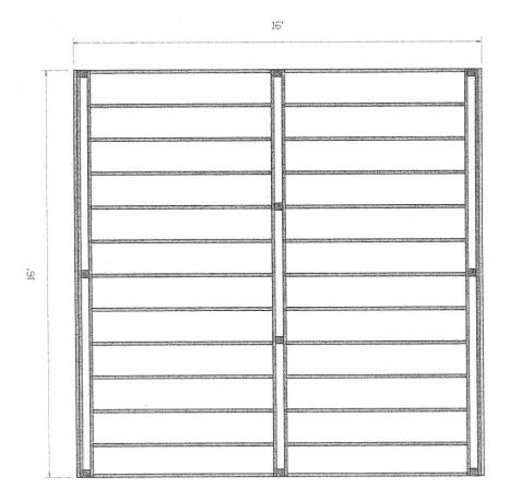
LOAD AND SUPPORT: Your deck will support a 69 PSF live load. Posts have 0" below-ground post support.
